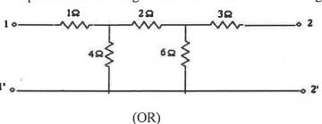
b) Determine the h parameters for the circuit shown in below figure.
