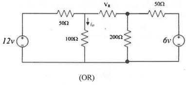
b) In the circuit shown in Figure determine the current Ix.
